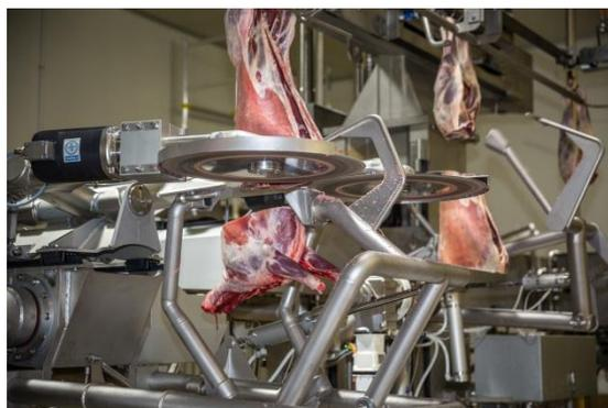
cutting machine then separates the carcass into hind, middles and forequarter cuts. A robot middles cutting machine then separates middles into racks, loin, flap or saddle. It's another example of our strategy to lift returns to farmer shareholders by improving the efficiency of livestock processing. It promises higher product yields with additional productivity and safety benefits.
